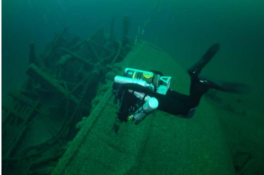
Figure 58. The *Floretta*'s starboard bow with the ground tackle and rigging visible. Tamara Thomsen.
