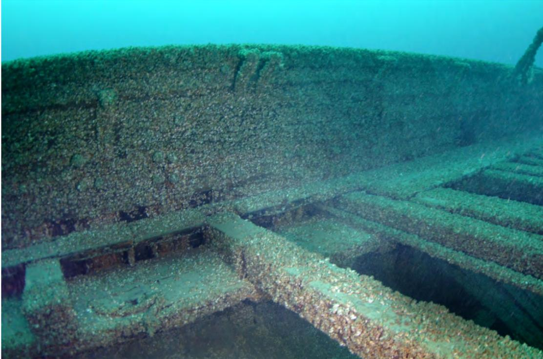
Figure 19. Deck beams have been removed throughout the hull. Looking to port at approximately amidship.
