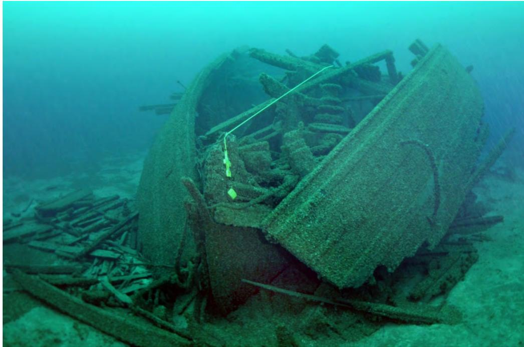
Figure 17. Broken bow with collapsed windlass deck.
