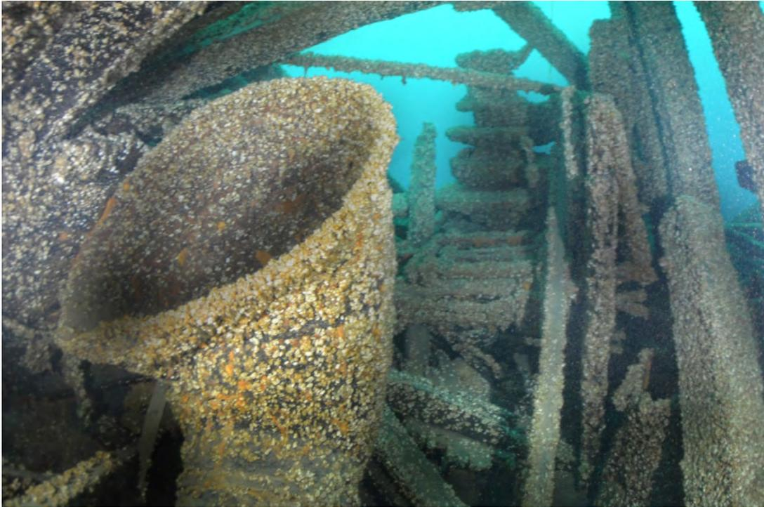
Figure 18. Large ventilation funnel lies below deck aft of the windlass, visible in the background.
