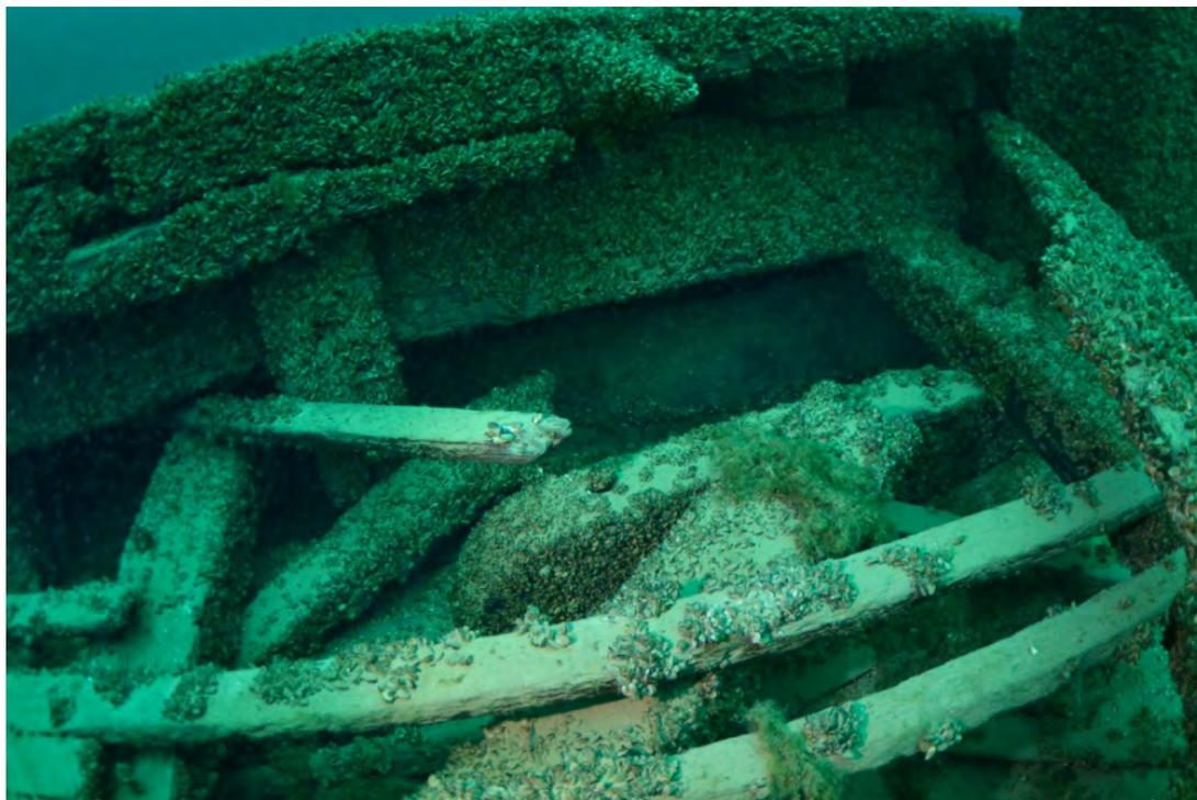
Figure 6. Reinforcing timber fastened atop the starboard side of keelson, aft of the centerboard trunk. A similar timber is fastened forward of the trunk on the port side of the keelson.
