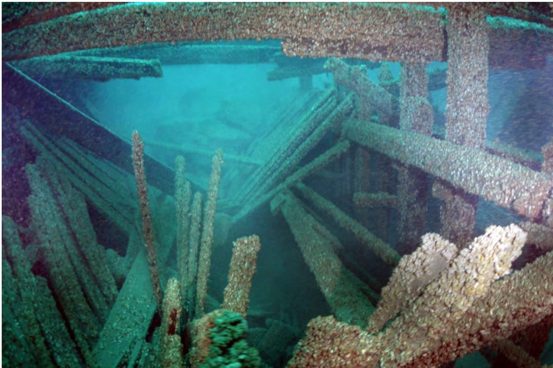
Figure 21. Collapsed section of port side hopper showing longitudinal timbers fastened to deck stanchions. Approximately amidship on port side, looking forward.
