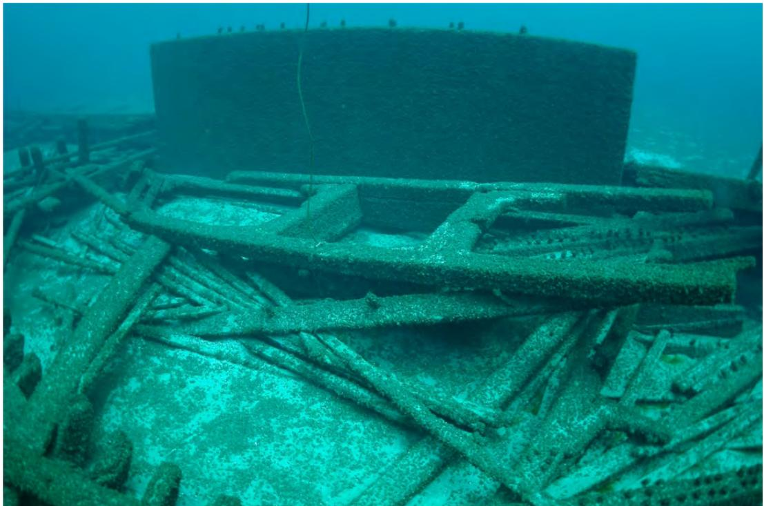
Figure 4. The center cargo hatch lies inverted along the starboard side of the centerboard trunk.
