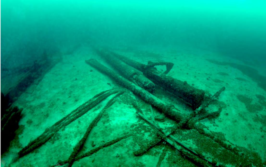
Figure 10. View of the mizzen- and mainmasts, looking forward from off the starboard quarter. The mizzenmast is on the right.
