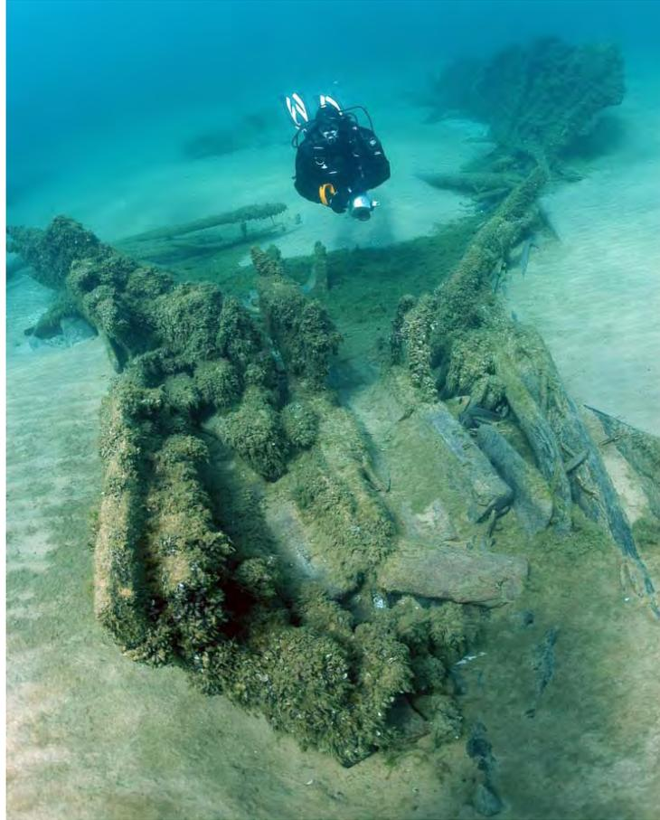
Figure 34. Vessel's stern, looking forward. Stern post is obscured by sand and algae, but shaft log is readily visible.
