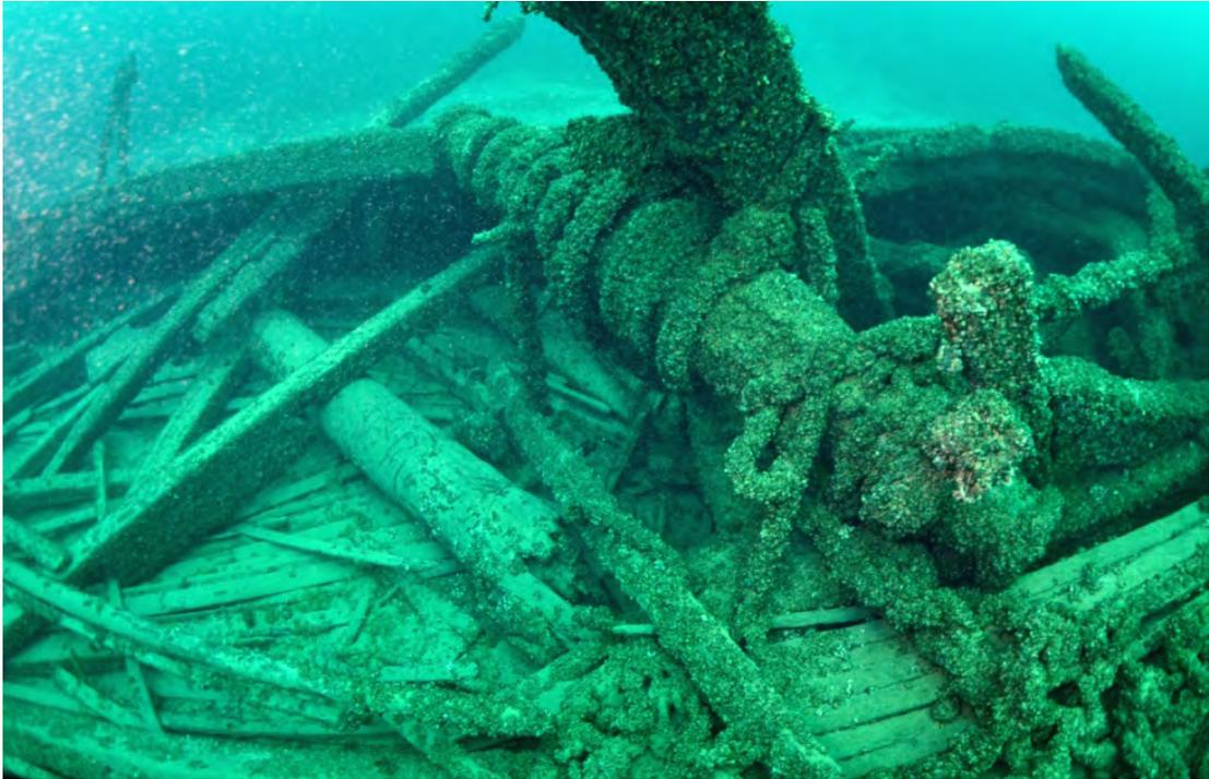
Figure 3. Windlass with norman pins. Base of foremast lies on floors aft of windlass.
