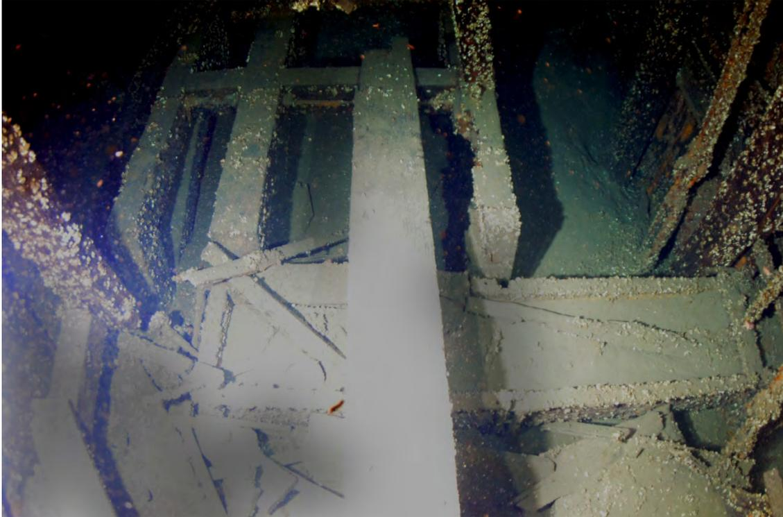
Figure 22. Intersection of port side longitudinal and athwartship conveyors.
