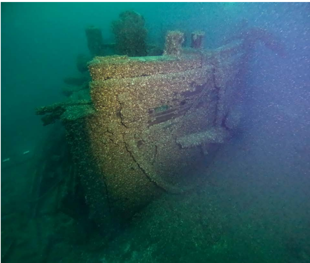
Figure 41. F.J. King 's stempost and port hull looking aft
