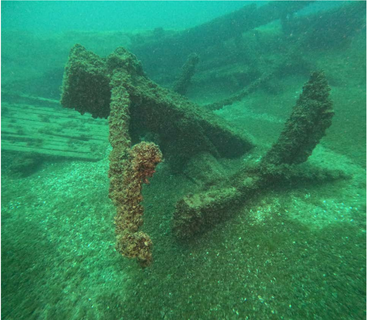
Figure 29. Thomas H. Smith 's Sampson post and windlass, looking from the starboard side across to the port side of the vessel.
