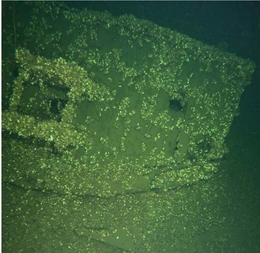
Figure 21. Jennibel's stern deck with steering carriage (Zach Whitrock)
