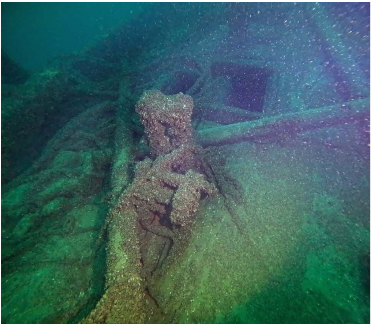
Figure 45. F.J. King 's centerboard winch and mainmast boom cradle
