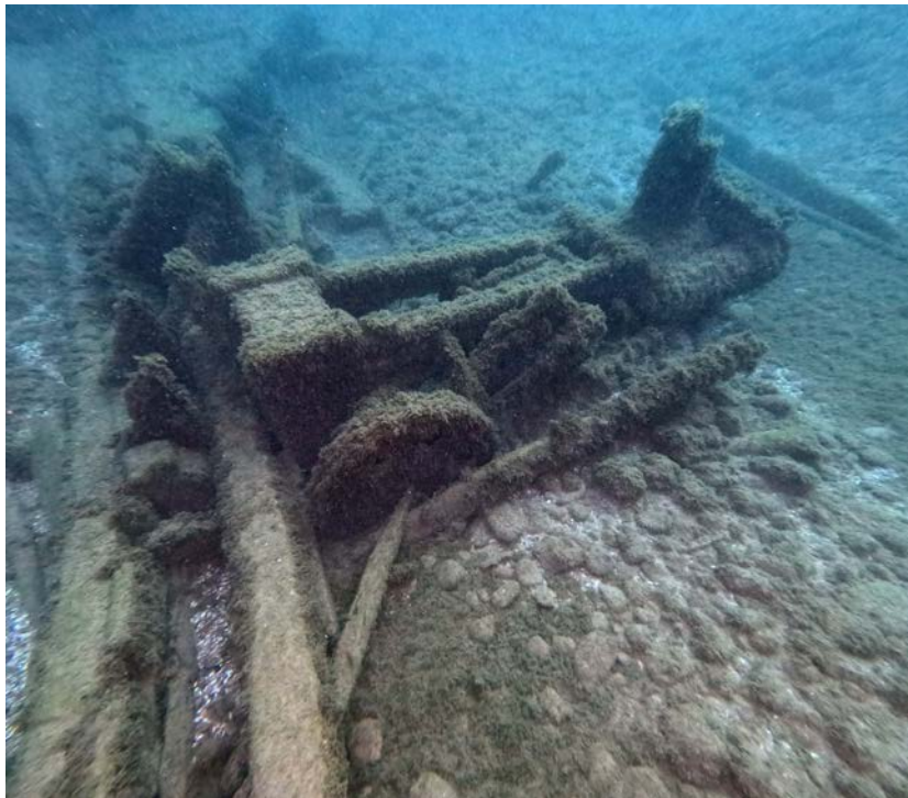
Figure 7. John Evenson's single cylinder, vertical steam engine
