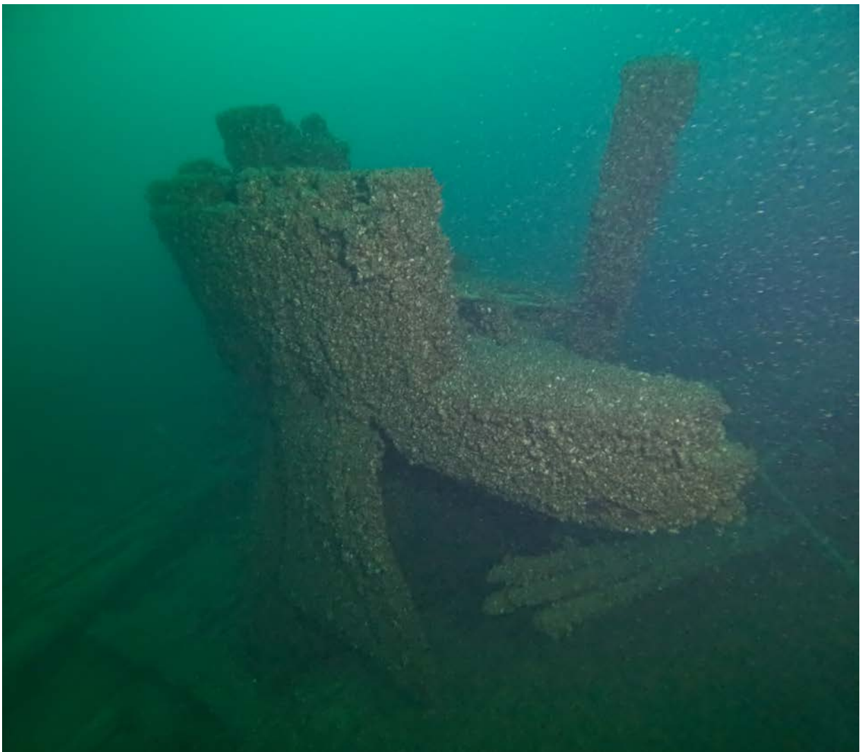
Figure 47. F.J. King 's stern with loose hanging lumber port cover
