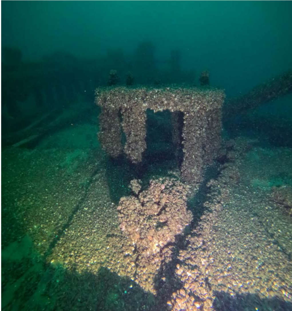
Figure 43. Lower portion of a single action bilge pump and foremast mast looking forward
