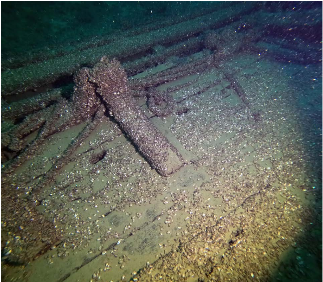
Figure 46. Port side of F.J. King 's disarticulated hull fragment with hanging knees and salt channels
