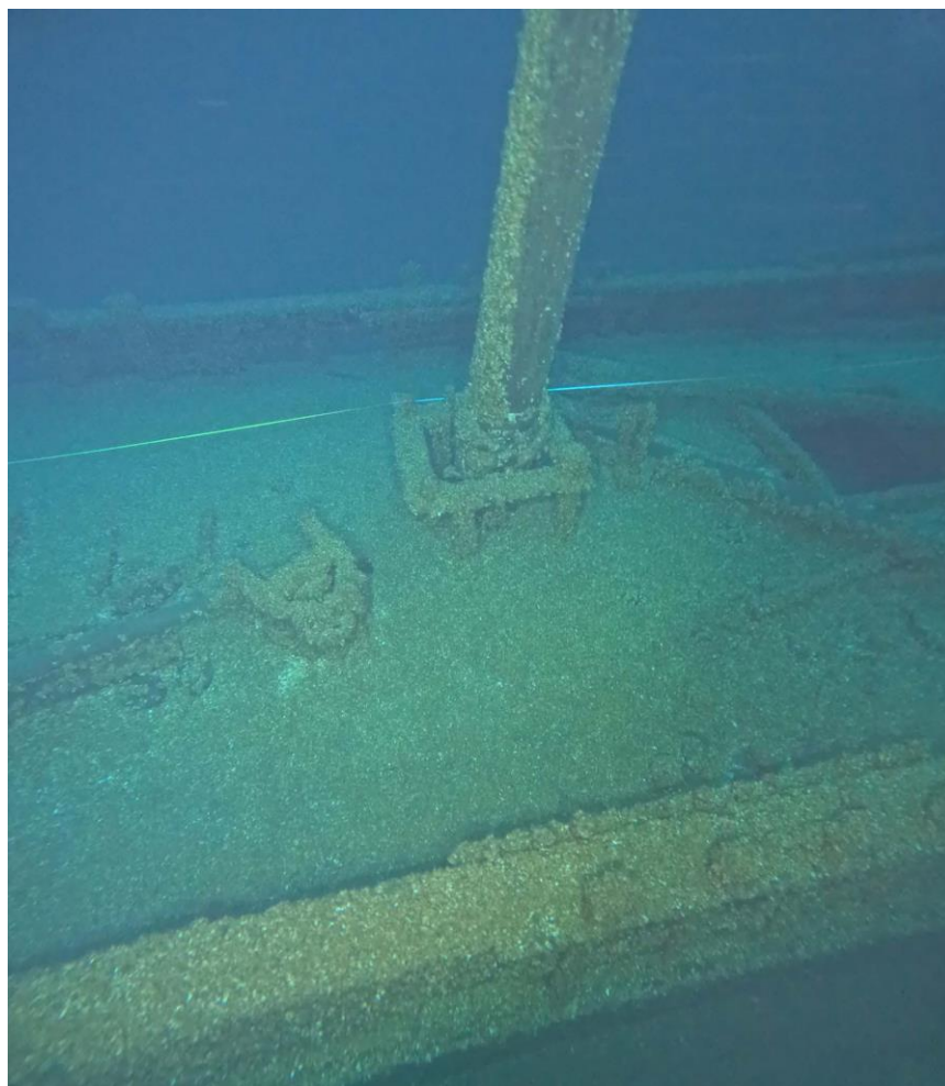
Figure 49. Mojave's upright mainmast with mast table. The centerboard winch toppled to starboard (Zach Whitrock)
