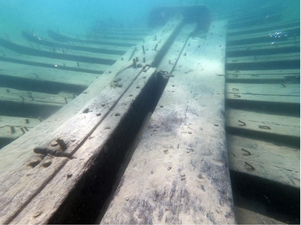
Figure 18. Grey Eagle's offset centerboard slot
