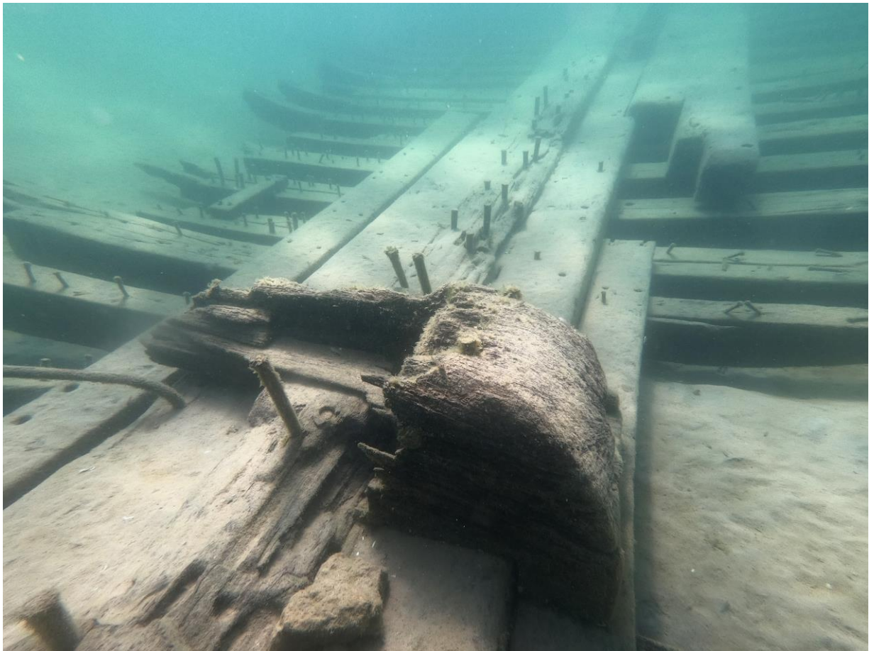
Figure 17. Grey Eagle's broken mainmast step
