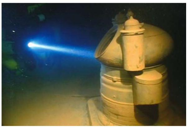
Figure 6. The binnacle on the forward deck of *Thomas Friant*, just forward of the pilothouse (Ken Merryman, GLSPS).
