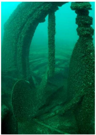
Figure 18. Selah Chamberlain's upright rudder and propeller (Wisconsin Historical Society).
