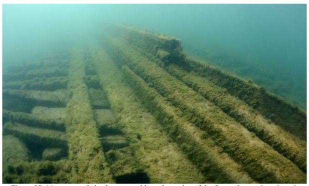
Figure 27. *Montgomery*'s keelson assembly and remains of the forward centerboard trunk (Wisconsin Historical Society).
