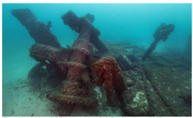
Figure 51. *I.A. Johnson*'s fallen samson post and windlass. Note the upright bilge pump in the background (Wisconsin Historical Society).
