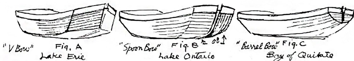
Figure 1. Various scow bow structures (Loudon Wilson).
