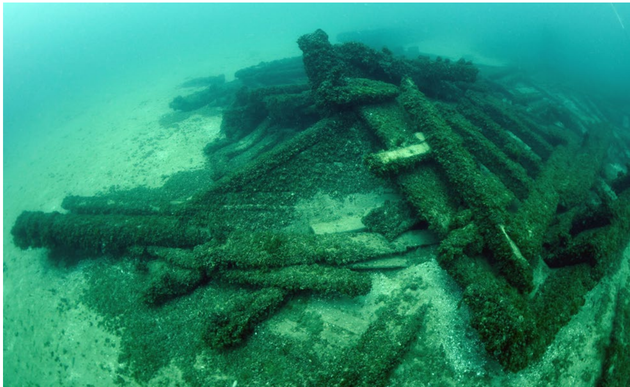
Figure 17. Flattened stern of I.A. Johnson showing cross planking and floor stringers/keelsons (Wisconsin Historical Society).
