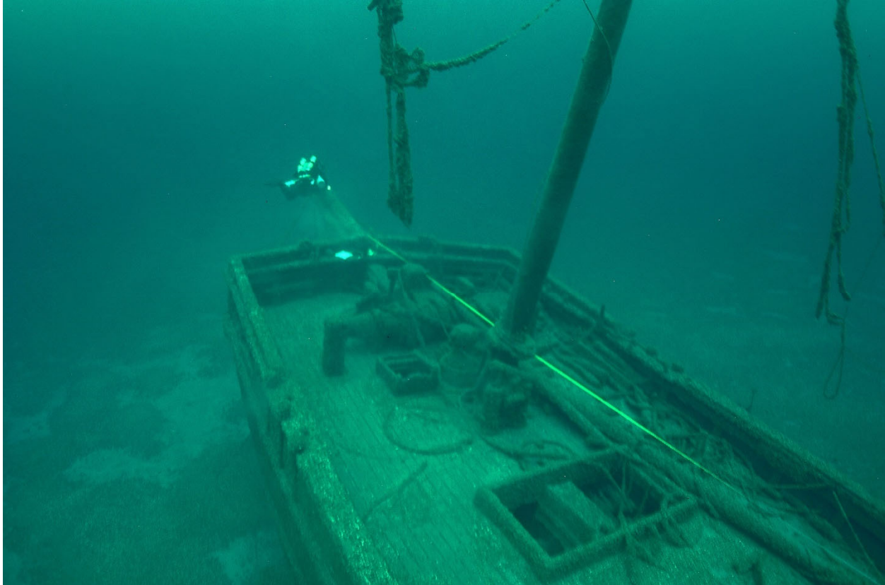
Figure 5.11. Bow and forward cargo hatch with visible portion of forward centerboard trunk, scow schooner Silver Lake (Wisconsin Historical Society).
