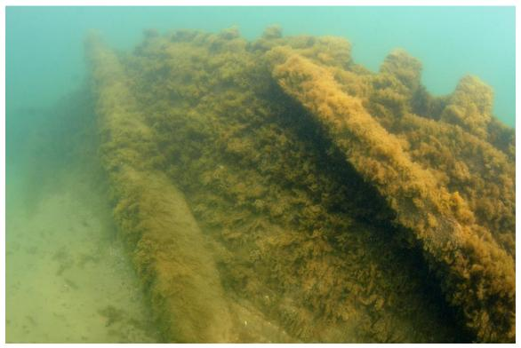
Figure 31. Wooden hogging trusses on the port side hull bow section
