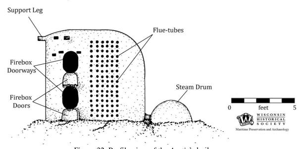
Figure 32. Profile view of the Arctic's boiler
