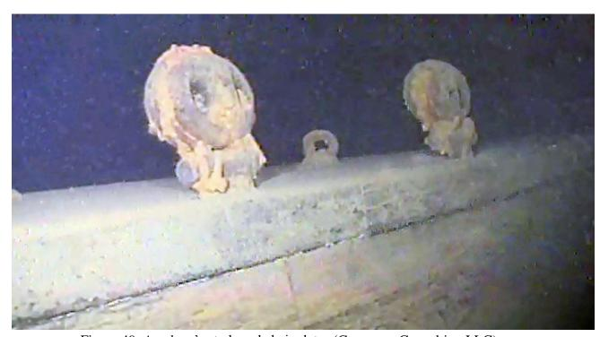
Figure 49. Antelope's starboard chainplates (Crossman Consulting LLC)
